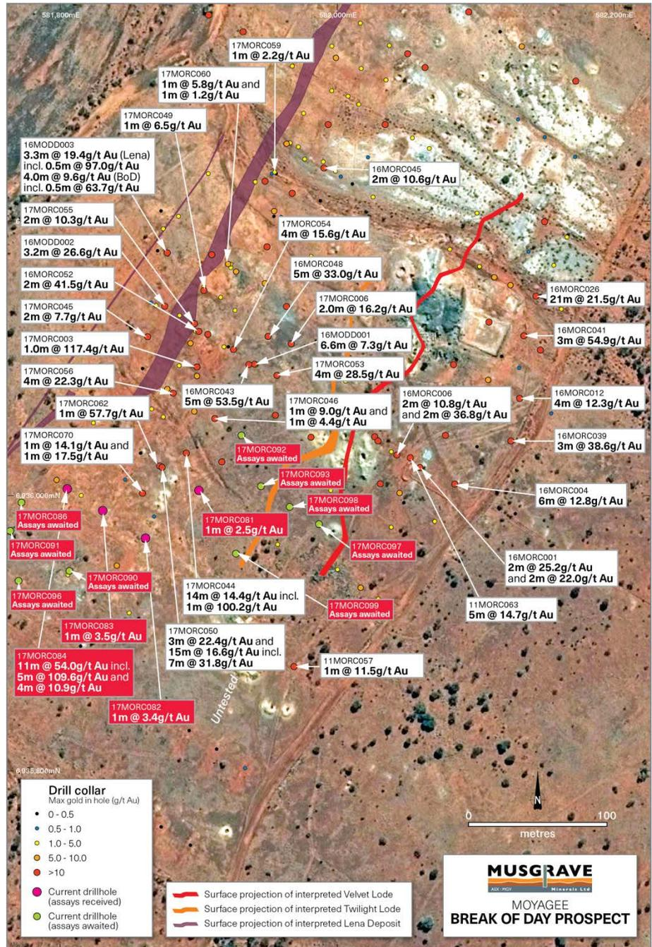
Figure 1: Location plan showing maximum gold in hole plotted at the drill hole collar and significant intersections for the Break of Day gold deposit
