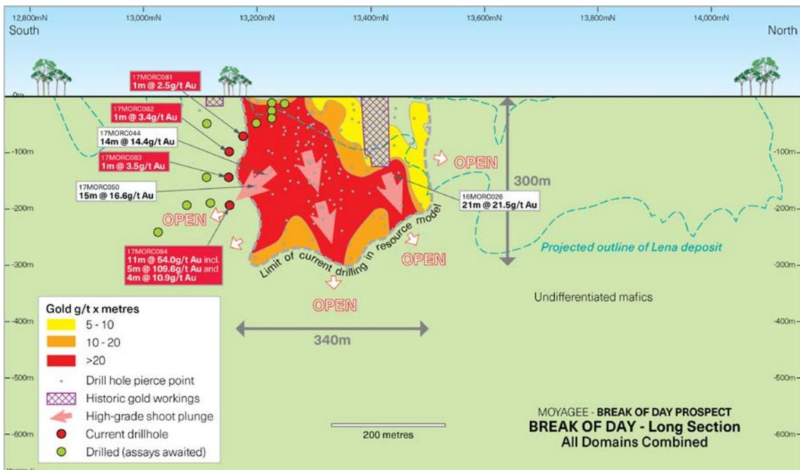
Figure 3: Break of Day schematic long section of the combined Twilight and Velvet gold lodes with new drill hole locations and the projected outline of the Lena deposit which is located approximately 130m west of Break of Day together with new drill target (a long section or longitudinal section is a section along the plane of the lode and in this instance shows gold grade x thickness variability with depth of the combined Lodes)
