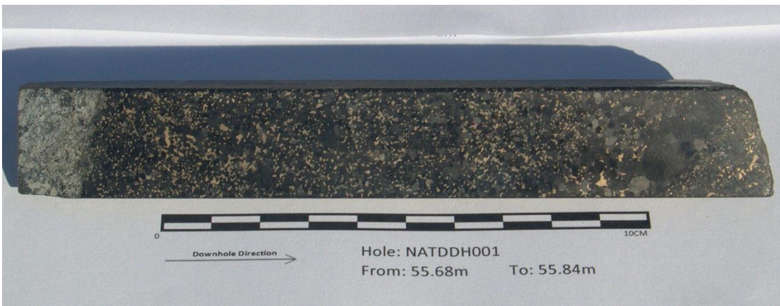
Figure 4: Example of Disseminated Sulphides in Drill Core at Na'Toth in NADDDH001 from Deering Hills
